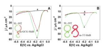
Figure 4: Current densities (a) after immobilization of the DNA-SL probe and 6-mercapto-1-hexanol (b) incubation with adaptor strands (m and f) and (c) incubation with m, f and target. Insets are computational modeling using NUPACK for **A**) m-GCG-MeB and **B**) m-3T-MeB.
